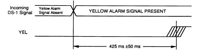
Figure 5 illustrates the assertion of the YEL output following the detection of an incoming Yellow Alarm signal. In SF and SLC®96 framing formats, the Yellow Alarm signal is transmitted by forcing bit 2 of every channel to zero. In T1DM framing format, the Yellow Alarm state is indicated by the Y-bit in the T1DM sync byte located in channel 24 of every frame. Yellow alarm is transmitted by setting the Y-bit to zero. In ESF framing format, Yellow Alarm is transmitted in the facility data
