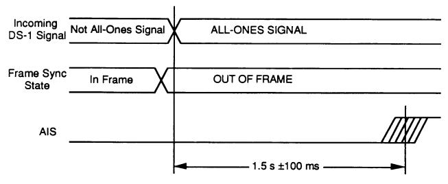
Figure 10 shows the assertion of the AIS output following the out-of-frame synchronization and the detection of the all-ones signal on the input.
