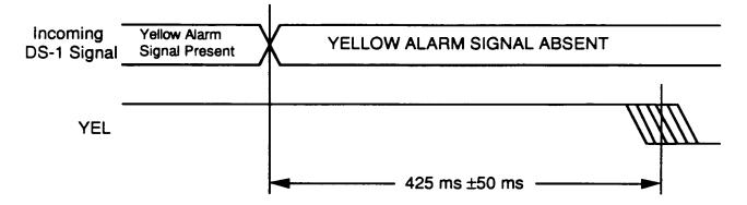
Figure 6 illustrates the deassertion of the YEL output following the detection of the lack of the Yellow Alarm signal in the input data data stream.
