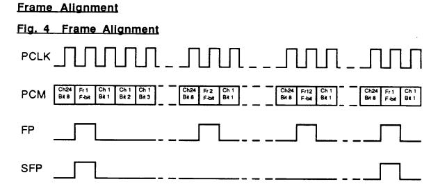
Figure 4 shows the relationship between the PCM clock (PCLK), the PCM data (PCM) and the framing pulses (FP and SFP) for the case where there are twelve frames per superframe (SF, SLC®96 and T1DM framing format). For the case where there are twenty-four frames per superframe (ESF framing format), the SFP pulse occurs every twenty-four frames (during the first bit of frame one) instead of every twelve frames.
