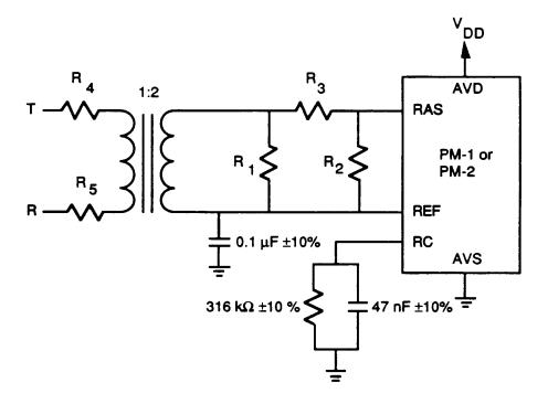
Terminate Mode Bridging Mode  $\begin{array}{lll} R_1 = 412 \ \Omega \pm 1\% & R_1 = 400 \ \Omega \pm 1\% \\ R_2 = 1.1 \ k\Omega \pm 1\% & R_2 = \text{Open Circuit} \\ R_3 = 9.0 \ k\Omega \pm 1\% & R_3 = \text{Closed Circuit} \\ R_4 = R_5 = \text{Closed Circuit} & R_4 = R_5 = 432 \ \Omega \pm 5 \% \\ \end{array}$
