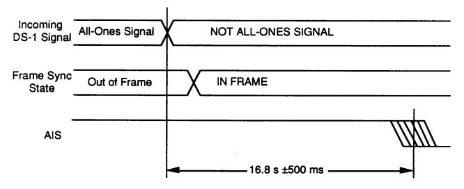
Figure 13 shows the deassertion of the AIS output after the all-ones signal has not existed on the input data.
