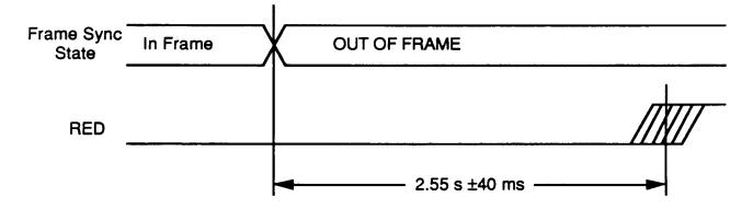
Figure 7 shows the assertion of the RED output following the out-of-frame.
