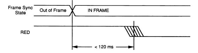
Figure 9 shows the "fast" deassertion of the RED output following frame synchronization. Fast deassertion mode is enabled by setting the FASTD bit of the ALMI Interrupt Enable Register to logic 1.
