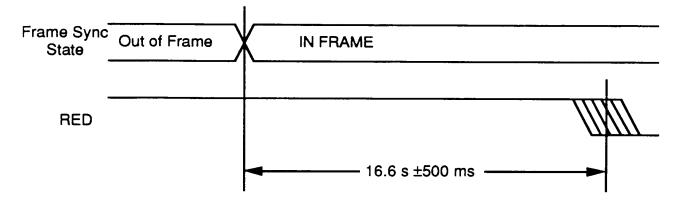
Figure 8 shows the deassertion of the RED output following frame synchronization.
