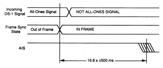
Figure 11 shows the deassertion of the AIS output following frame synchronization.
